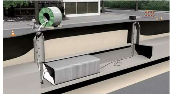
Example of “trenchless” system (SPR)
